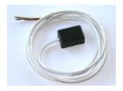
The SensoPad is an interface used to send an output contact to any interactive device. It is a proximity sensor which does not require direct contact. Stuck onto an insulating material, the SensoPad detects presence of a finger, or any other trigger, through the material.
