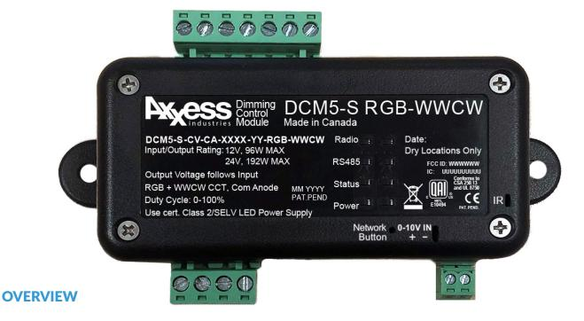
The DCM5-S, RGB+CCT (aka RGB WWCW) is a compact 5 channel, low side, LED Controller, designed to be interfaced with power supplies ranging from 12VDC to 24VDC.
