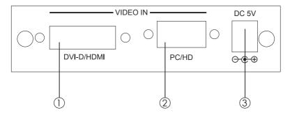
① DVI-D/HDMI: Connect the PC input DVI (29 pin) port to the DVI-D/HDMI output port of your HDMI source equipment such like PC.
