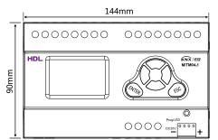
Figure 2. Dimensions - Front View
