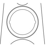
Hold the ring by one of the indentations by depressing the grille fabric with your thumb, and then wiggle the ring forwards until it comes free of the speaker. The grille fabric is very resilient and any depressions will soon disappear.
