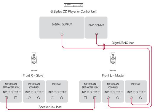
If the Meridian source or control unit provides a Meridian BNC Comms output, you will need to connect it to the DSP Loudspeakers using a Digital/BNC lead.
