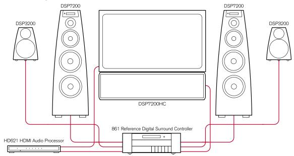
Up to eight Meridian DSP loudspeakers can be used in conjunction with a Meridian surround controller, such as the 861 Reference Digital Surround Controller, to create a digital surround system with superb music and cinema sound. The HD621 integrates HDMI switching seamlessly into a Digital Theatre system, separating the audio from the video stream and allowing the best possible audio playback from HDMI sources.
