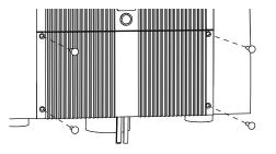
Connect the loudspeakers as required (see *Connecting the loudspeakers*, page 16), then lead all the cables neatly through the slot in the base of the cabinet:
