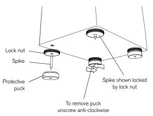
On carpeted floors all parts can be fitted and the spike should be adjusted so that it extends through the puck and penetrates the carpet pile to the floor underneath. Where a carpet has a deep pile you can fully unscrew and remove the puck to expose more of the spike.
