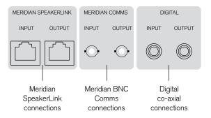
You can connect to the DSP loudspeakers using either the SpeakerLink connectors, or the Meridian BNC Comms and digital co-axial connectors.
