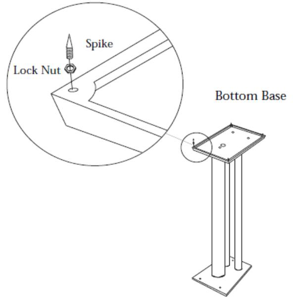
**Step 5-** Place your Revel Concerta2 M16 loudspeaker as shown onto a carpeted surface or a soft towel. Attach the assembled stand with four 1/4x20 x 1.0" Phillips head screws.
