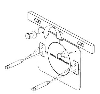
Level & pin template to wall. Sub can be positioned horizontally (landscape) or vertically (portrait) with binding posts at either end. Outline wire hole and all 8 screw holes for 2 mounting posts. Screw post(s) into a stud if possible.
