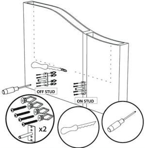
Cut wire hole; install anchors if there are no studs. Always screw both mounting posts to wall with 4 screws per post. Test both posts for shear strength.
