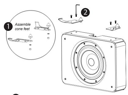
1: Attach cone feet to the standing feet with acorn nuts & washers (see insert). 2: With cone feet to the back of the enclosure, securely screw the 2 standing feet into the 4 inserts in the bottom of the enclosure with 4 button screws and 5/32" Allen key.
