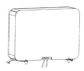
Securely connect speaker wires (min 14 gauge AWG) through push-in binding posts. Be sure to preserve correct polarity with amp (red to red).
