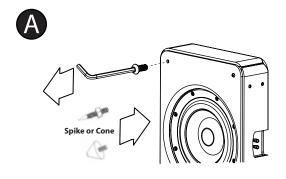
With grill off, remove all 4 button screws from enclosure face with Allen key; replace with included spikes or cone feet. Adjust so that all 4 feet make solid contact with floor or carpet without rocking or tipping. With spikes, remember to tighten the lock nuts.
