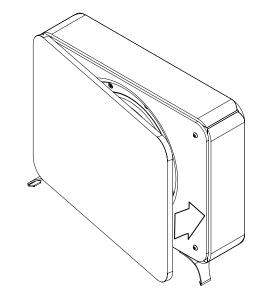
Attach grill at one end; snap grill into place making sure that all 4 magnets are secure and that grill is snug all around.
