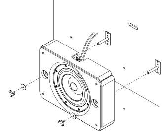
Attach adhesive backed bumper to each of the 4 back corners. Mount speaker on posts; loosely tighten knobs through washers into posts. Level or align +/- 1/4" (6.35mm), then tighten both knobs.
