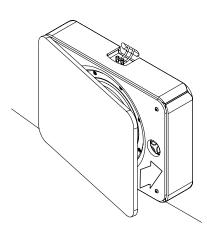
Attach grill at one end; snap grill into place making sure that all 4 magnets are secure. Snug all around. Connect speaker wires to RackAmp and set up RackAmp with instructions on Page 1.
