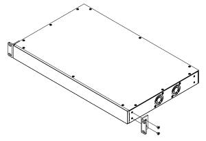
**Note:** Rack ears can be installed to the front or the back of the amplifier as needed.
